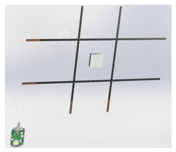
The mechanical design consists of two parts: the electronics housing and the pressure plate. For the housing an off-the-shelf enclosure was used from OKW enclosures. The part number is in the bill-of-materials at the end of the document. This housing also includes cut-outs for the LEDs, user button, and USB port and a cable gland to hold the wires from the pressure plate in place.
