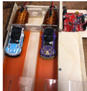
Figure 7. Close-up picture of electromagnet holders and beginning of track that I worked on.
